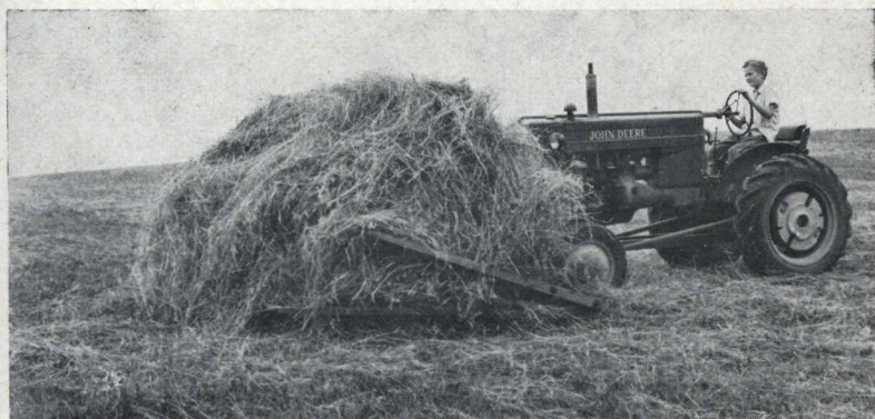
Fig. 36—Tractor-mounted sweep rake with hydraulic control, and a high forward speed, is loaded directly from the mower swath by double piling.
