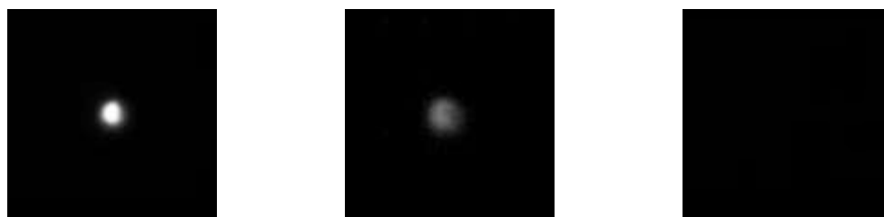
Figure 6.1. CCD camera images to show evidence of trapping of a fluorescent particle. Left: particle is trapped. Middle: particle is about to escape the trap (escape is along the Z-axis so that the image is defocused). Right: particle has fully escaped from the trapping region.
