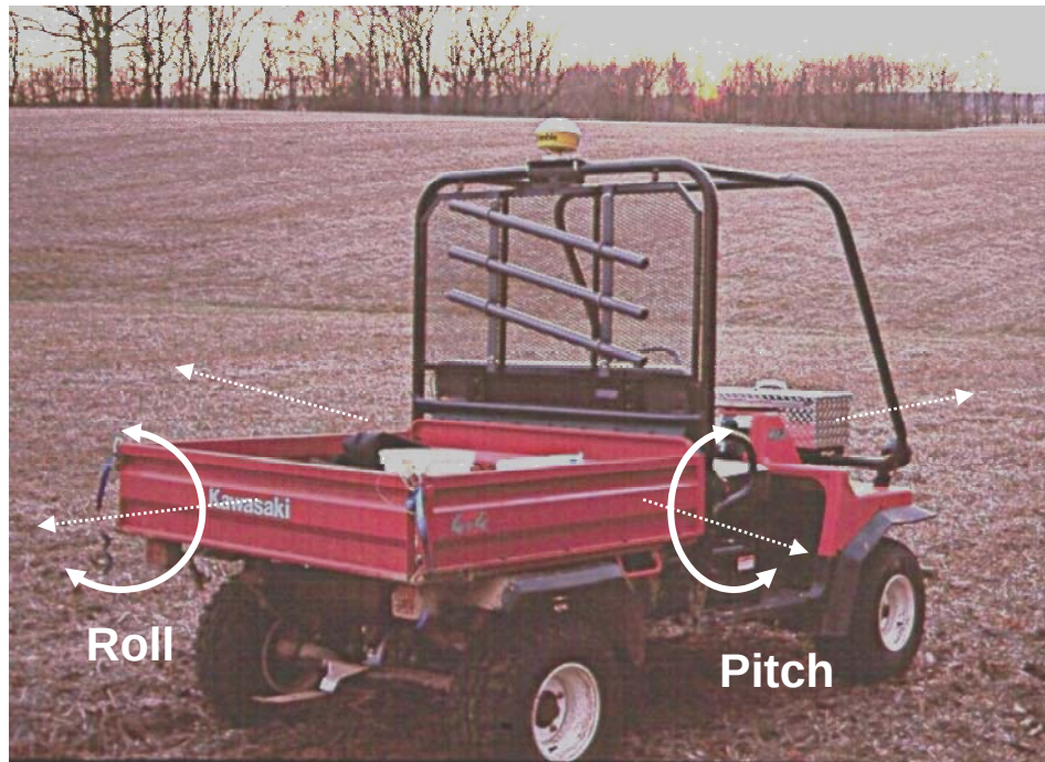
Figure 2. Pitch and roll angles of a vehicle.
