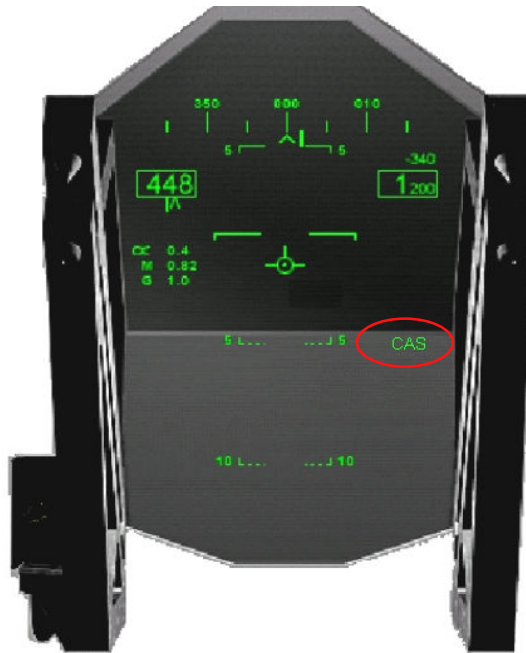
Figure 2.16; Placement of the VMF message cue
