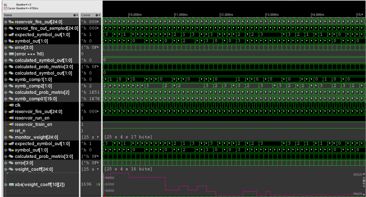
Figure 6.6: The simulation results from the Output Layer module offer valuable insights into the training dynamics of the neuromorphic architecture, with a specific focus on the evolution of weight coefficients throughout the training period.
