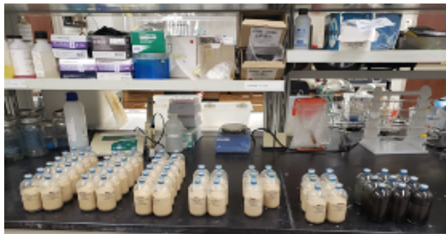
Figure 50. Microcosms established with aquifer slurries and composite groundwater or RAMM.
