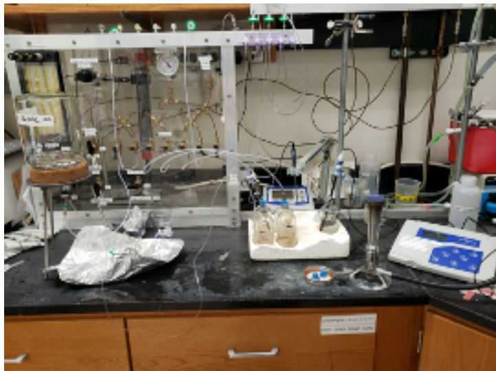
Figure 49. Dispensing of synthetic, defined reduced anoxic mineral salt medium (RAMM) to the glass serum bottles containing the composite slurry.
