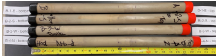
Figure 47. Aquifer material cores that were received prior to separating the cores into lower (bottom) and upper (top) cores.
