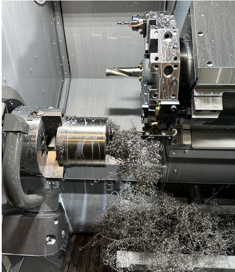
Figure 1.2: Birds nest created during boring operation on CNC lathe
