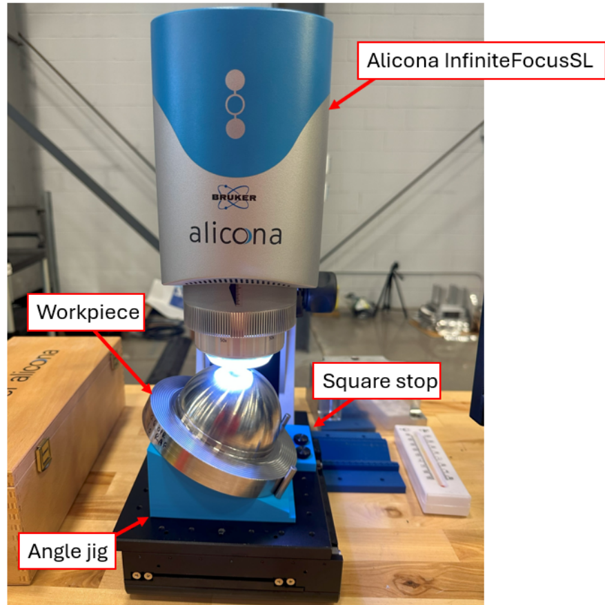
Figure 9.3: Alicona InfiniteFocusSL measurement setup with MTTP, angle fixture, and square stop.
