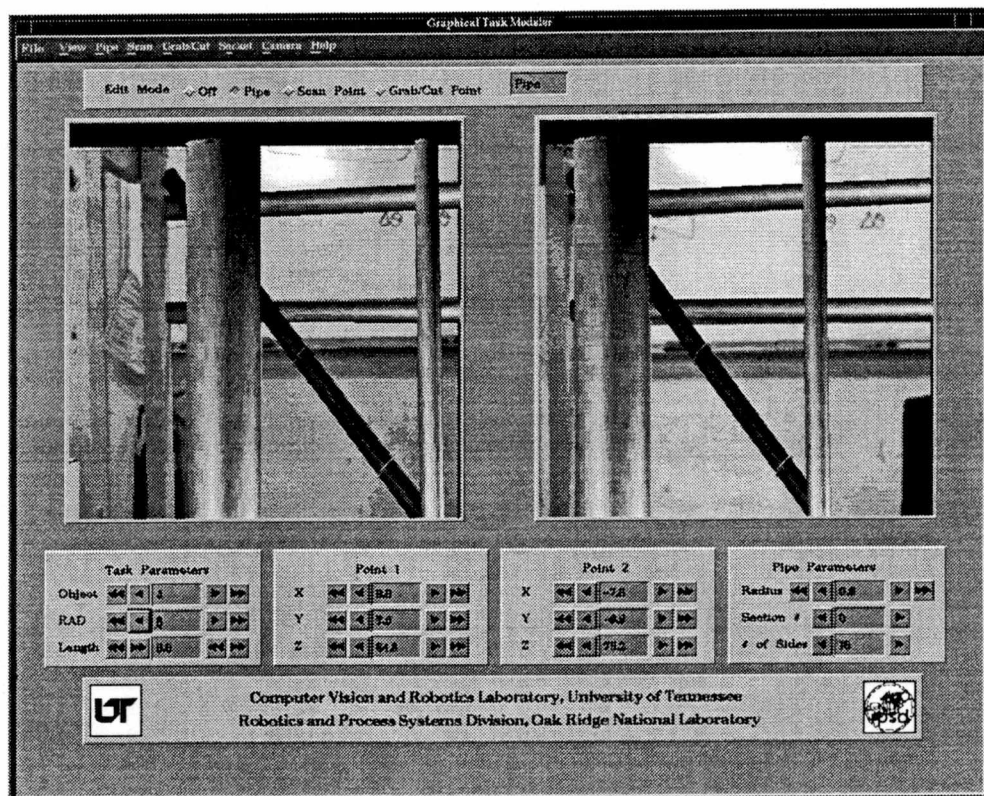
Figure 8.19: Models created from the integrated system with the stereo cameras mounted on the mobile platform.
