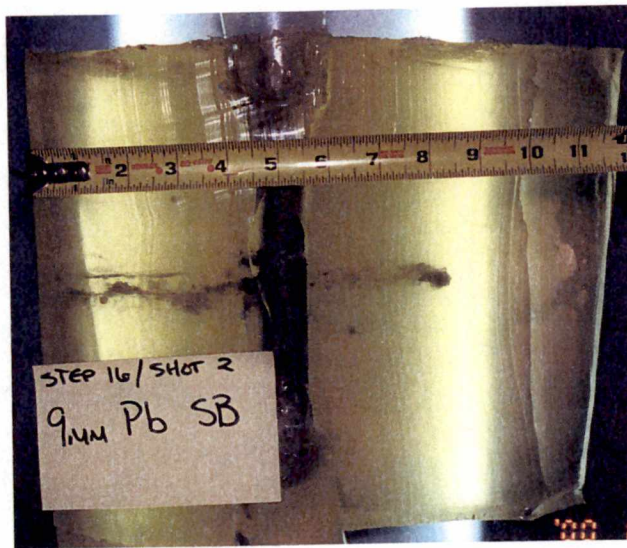
Figure A-27: Second lead pistol shot against a synthetic bone target.
