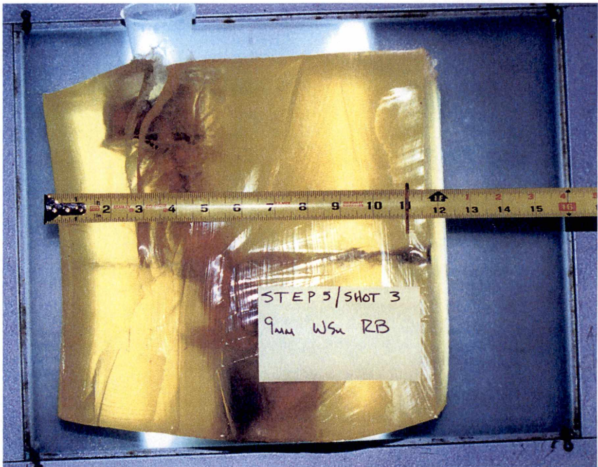
Figure 3-1: Tungsten tin pistol shot showing the trail of tungsten tin powder post-bone.
