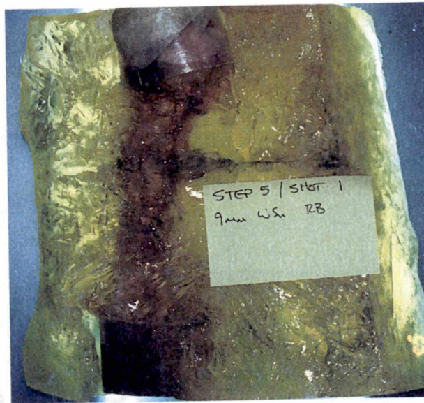
Figure A-7: First tungsten tin pistol shot against a real bone target.
