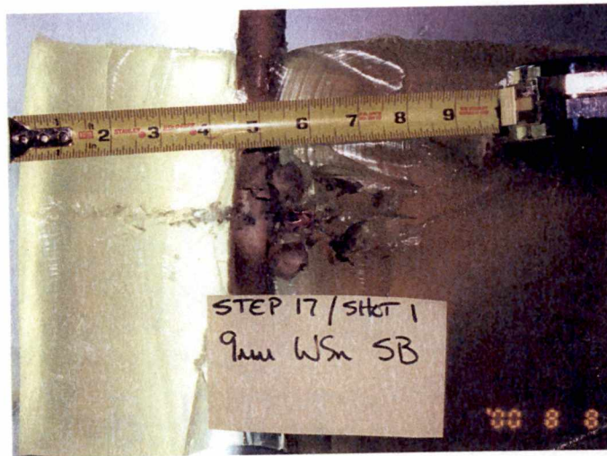
Figure A-31: First tungsten tin pistol shot against a synthetic bone target.
