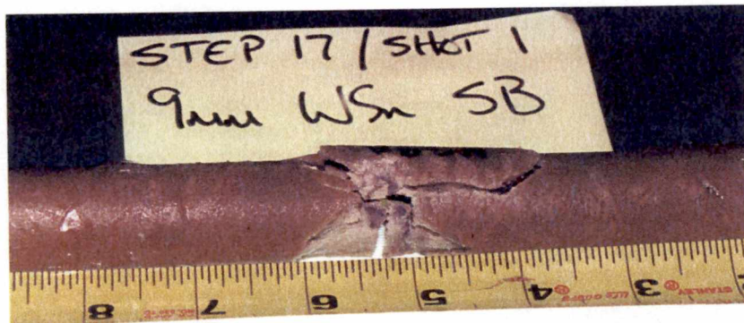
Figure A-32: Closer view of the synthetic bone from third lead pistol shot.
