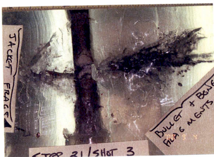
Figure A-48: Closer view of the synthetic bone from third tungsten tin rifle shot. Note again the comet-like dispersion of bullet fragments past the bone.
