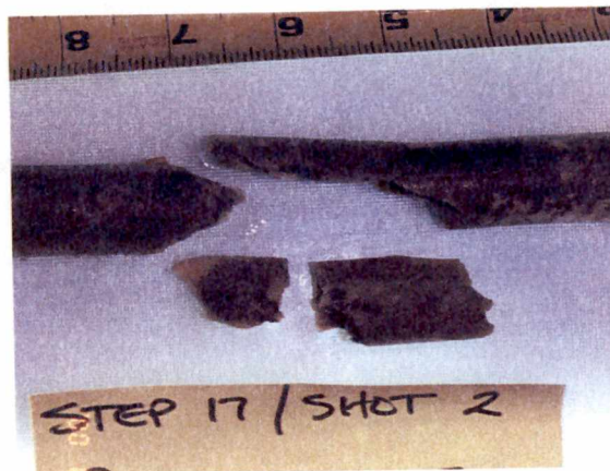
Figure A-34: Closer view of the synthetic bone from second tungsten tin pistol shot.
