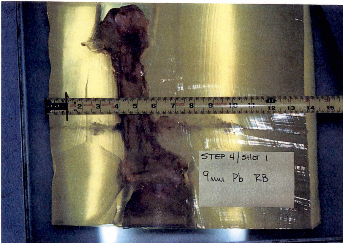
Figure 3-6: Lead pistol bullet target showing bone fragments in the permanent cavity immediately after the bone.
