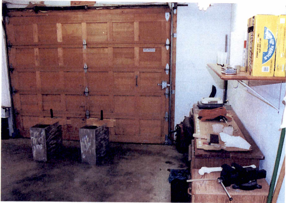
Figure 1-1: Photograph of the mold preparation room. The hot plate and mixing drill can be seen on the bench against the right wall. The two molds can be seen in bottom left of the photo.
