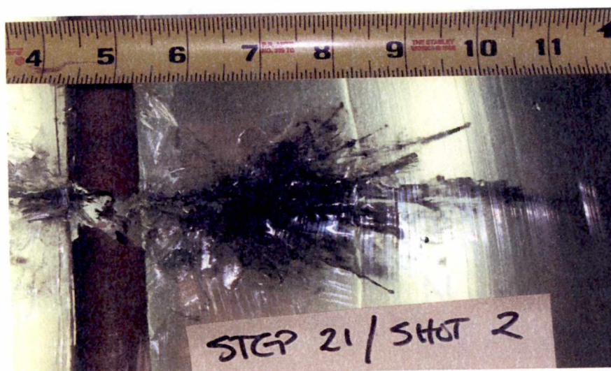
Figure A-46: Closer view of the synthetic bone from second tungsten tin rifle shot. Note the comet-like dispersion of bullet fragments past the bone.
