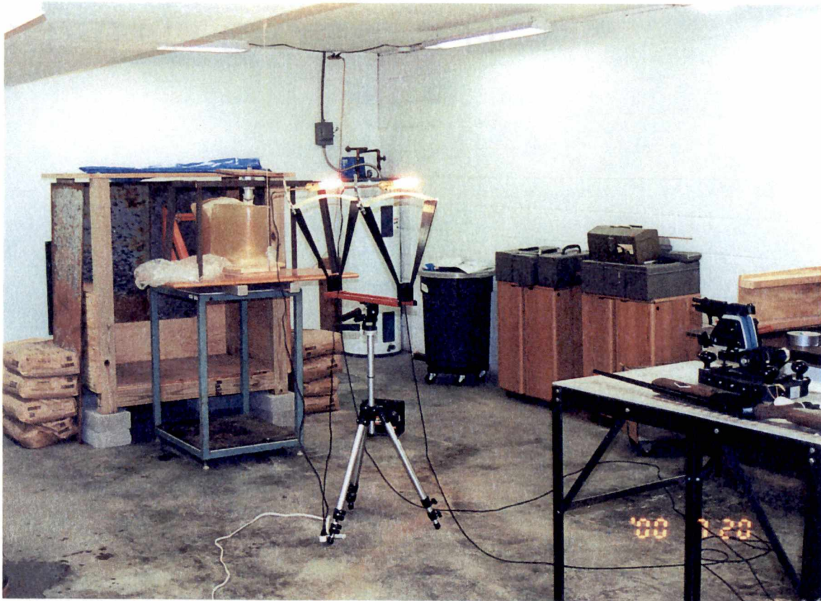
Figure 1-2: Photograph of the shooting area. The pistol stand can be seen in the lower right hand corner. The chronograph is in the center of the photo, and the target stand is in the right-hand side of the photo behind the chronograph. The bullet trap is the large wooden box behind the target stand.
