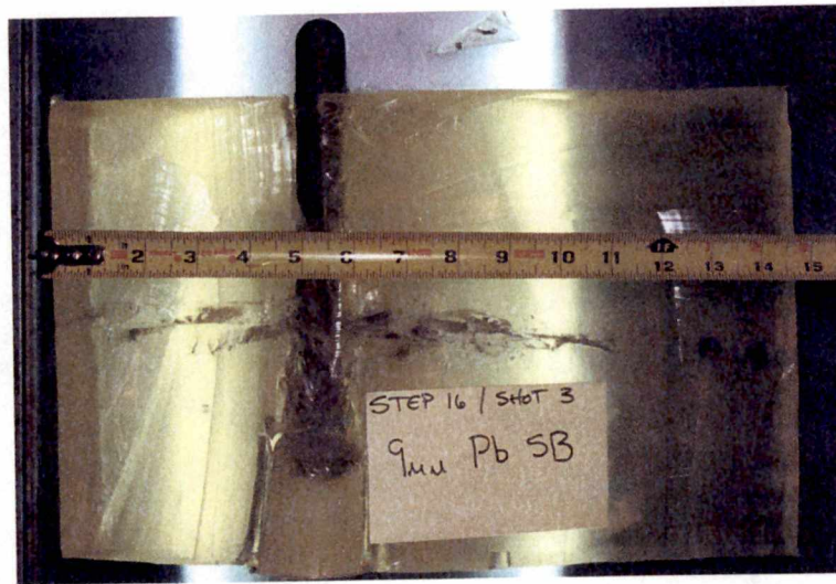
Figure A-29: Third lead pistol shot against a synthetic bone target.
