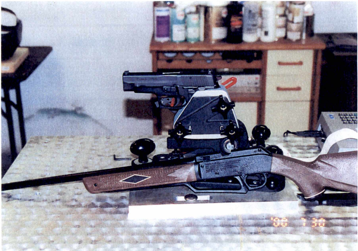
Figure 1-3: Photograph of the 9mm SIG-Sauer P-226 in the Ransom pistol rest. Also seen below the pistol is the Daisy Model 880 BB rifle used to calibrate the gelatin.
