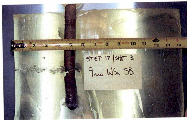
Figure A-35: Third tungsten tin pistol shot against a synthetic bone target.
