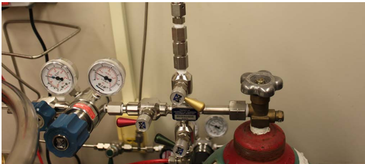
Figure 23. Photograph of Cross purge assembly with attached high purity regulator
