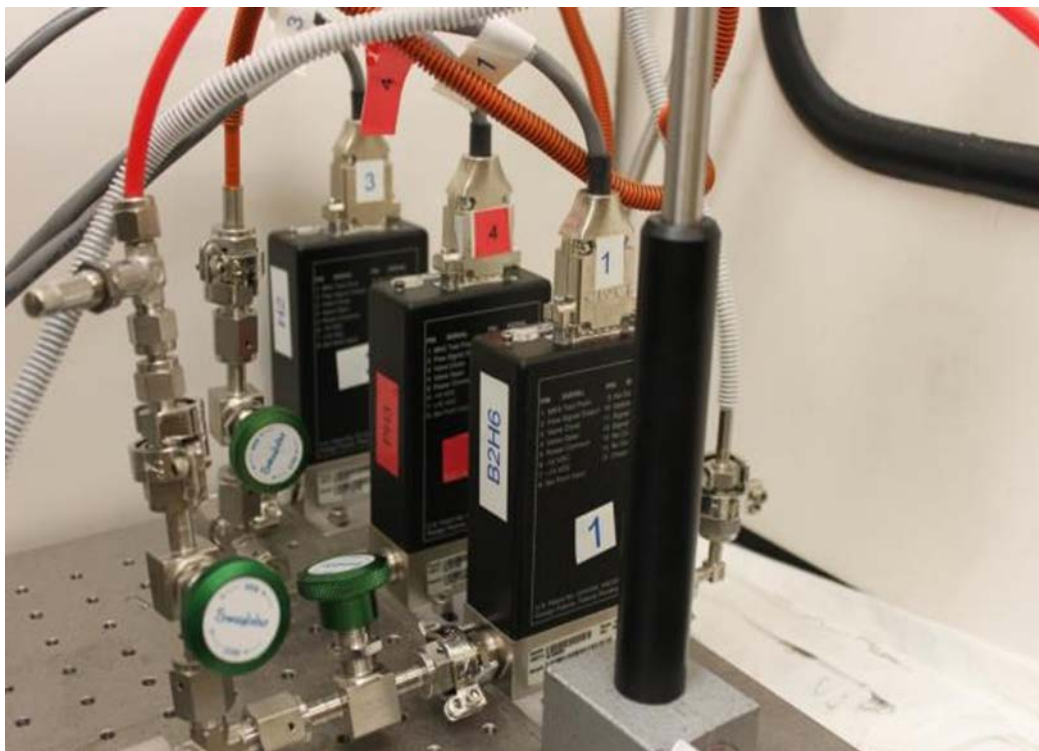
Figure 26. Photograph of MKS 1479A Mas flow controllers for diborane (front) Phosphine (middle) and Hydrogen (rear)
