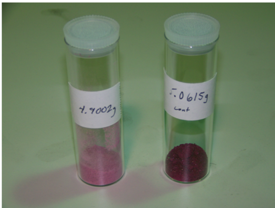
Figure 3.5: Ground (left) and un-ground (right) samples of hydrated cobalt chloride.
