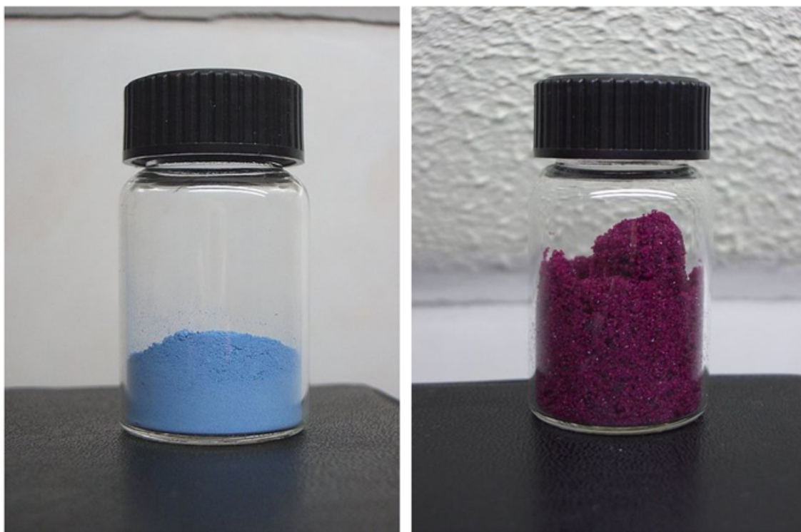
Figure 1.1: Anhydrous (left) and fully hydrated (right) cobalt(II) chloride [1].
