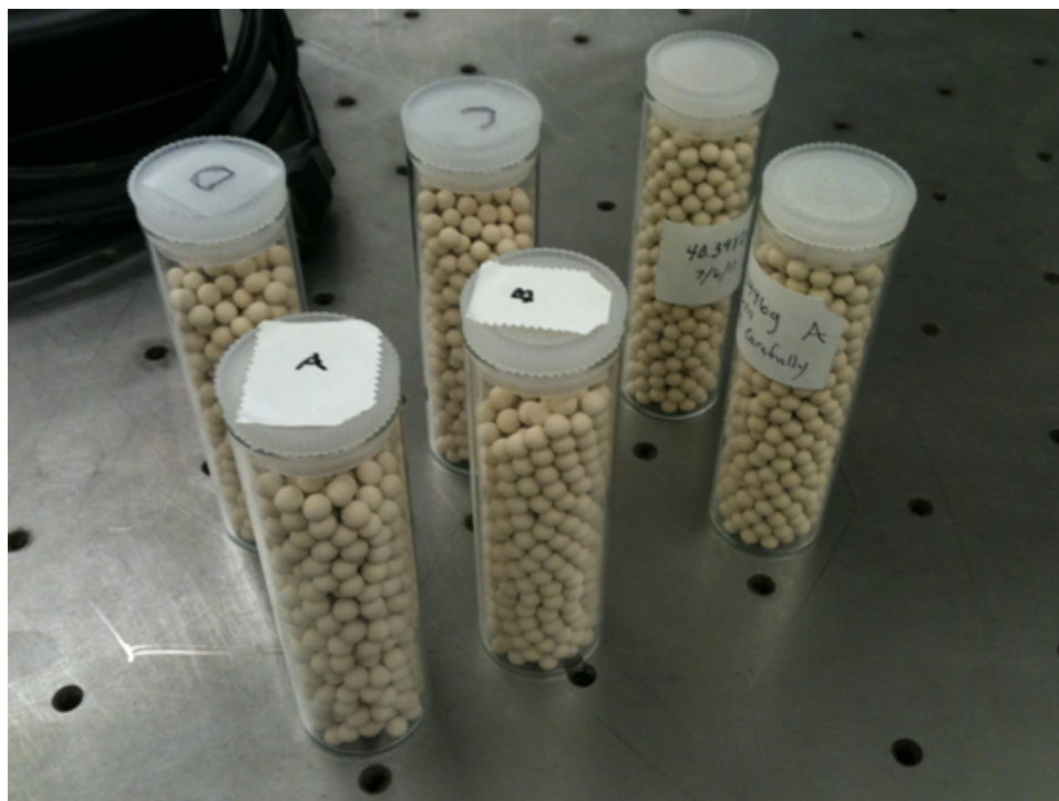
Figure 3.9: Photograph of 3Å K type zeolite molecular sieves.
