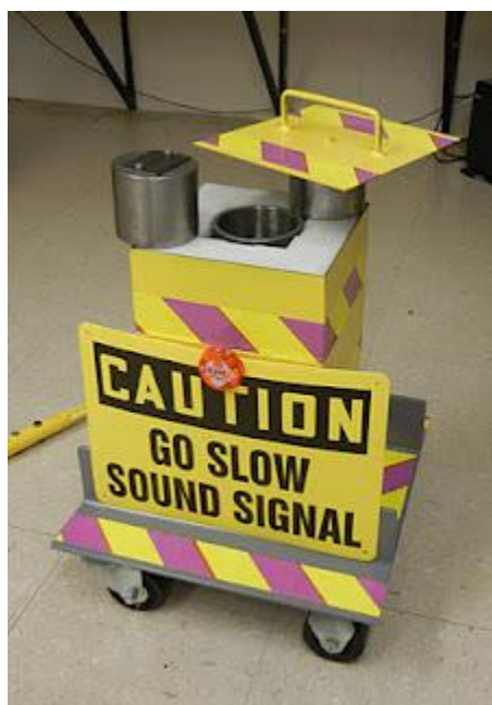
FIGURE 5 - CONSTRUCTED GAMMA IRRADIATOR
