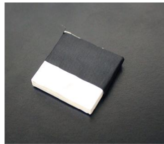
B - Single ^6\text{LiF} loaded ZnS:Ag Sheet (1.4" x 1.4") wrapped in Teflon tape (white), and gaffer tape (black).
