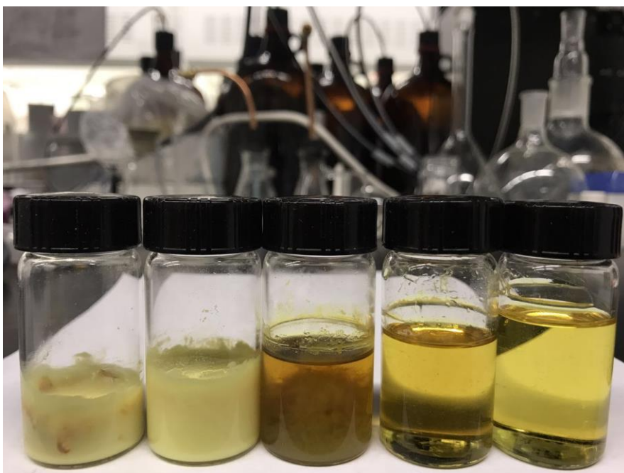
Figure 9.1 Polymerization occurred in DMF solvent (1mmol 4,4'-(9-fluorenylidene)dianiline with 1mmol terephthalaldehyde per trial)
