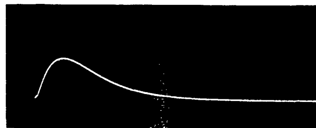
(h) Shaping amplifier output pulse without positive feedback and with shaping time constants of 4 \mu sec. (5 V/Div., 5 \mu sec./Div.)
