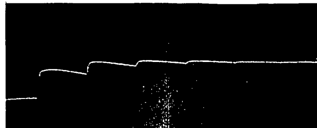
(b) Preamplifier output pulse without positive feedback. (0.5 V/Div., 0.2 \mu sec./Div.)
