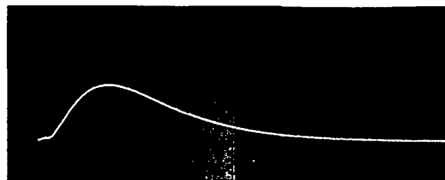
(f) Shaping amplifier output pulse without positive feedback and with shaping time constants of 1 \mu sec. (5 V/Div., 1 \mu sec./Div.)
