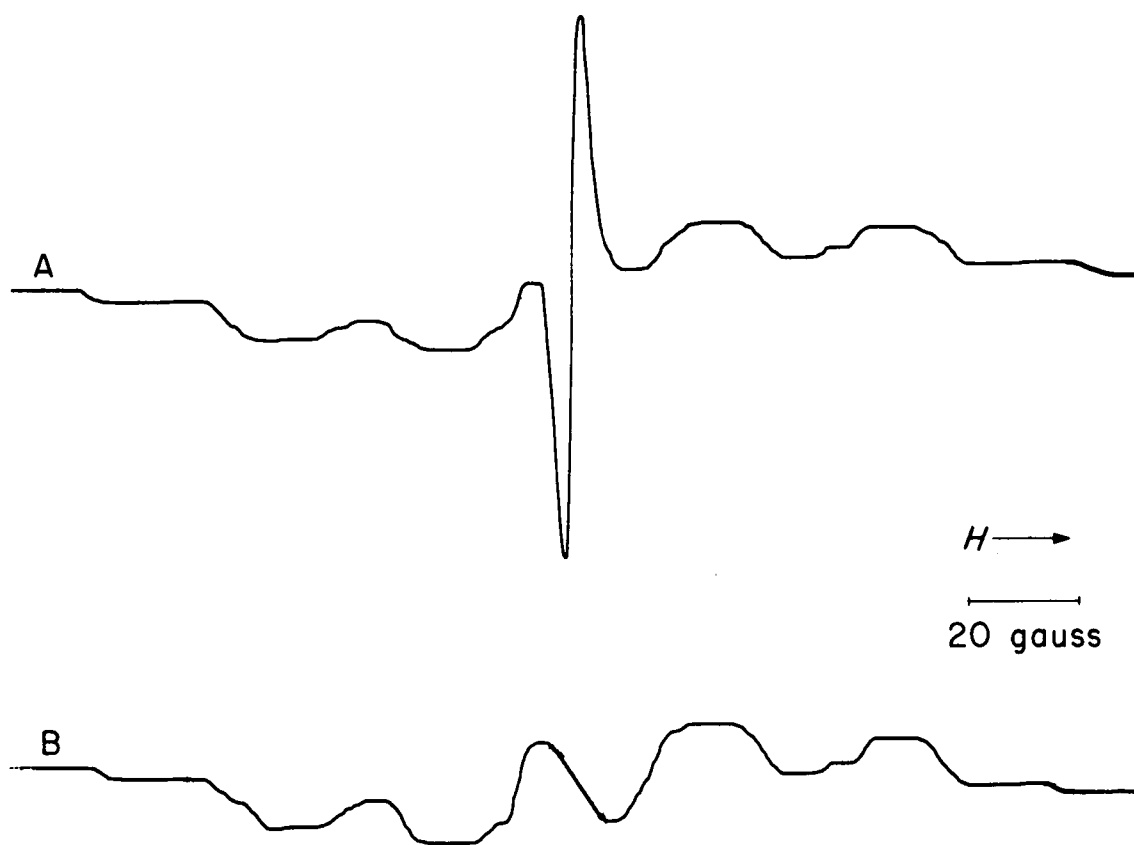
Figure 5. First-derivative ESR spectra of \gamma -irradiated antioxidant-free Marlex 6050 polyethylene at 77°K.
