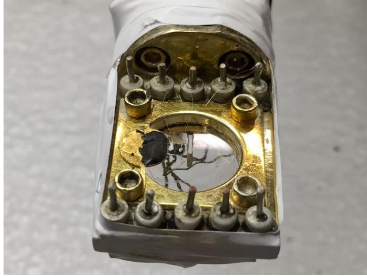
Figure 3-4: Prepared sample installed on sample stage.
