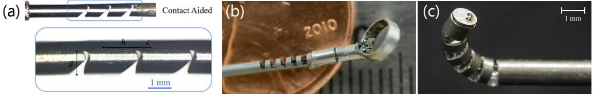
Figure 1.3: Examples of notched tube-based continuum robots with offset backbones. (a) is from [26], (b) is from [51], and (c) is from [25].
