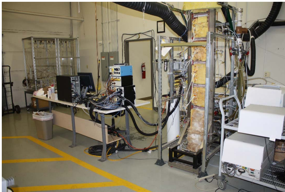
Figure 38: Plasma Oxidation Multiple Tow Reactor 1 (MTR1) using remote exposure.
