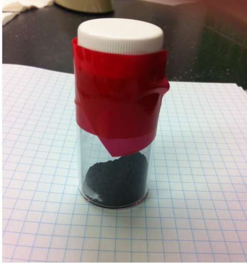
Figure 3.2: Shown here is a photo of the one of the \text{PrFe}_{1-x}\text{Ru}_x\text{AsO} powder samples. This vial contains about 2g of \text{PrFe}_{0.9}\text{Ru}_{0.1}\text{AsO} .
