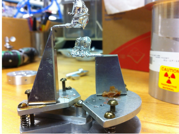
Figure 5.3: Two separate pieces of US single crystal wrapped in aluminum foil and mounted on aluminum brackets after alignment at the CG1 instrument of HFIR.
