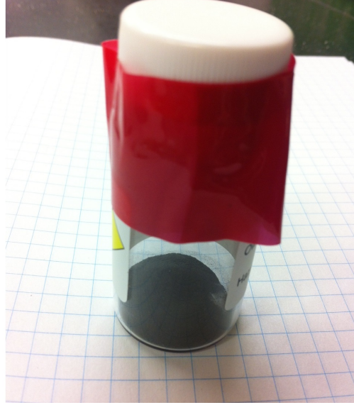
Figure 4.4: Shown here is a photo of the one of the \text{Fe}_{1-x}\text{Cr}_x\text{Ge} powder samples. This vial contains about 4 g of \text{Fe}_{0.97}\text{Cr}_{0.03}\text{Ge} .
