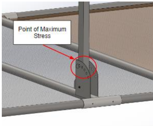
Figure 20: Safety Pin shear tear-out and supporting equations
