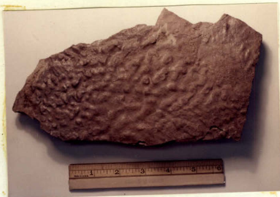
Figure 20. Flow casts from the Rome formation. A. Specimen from Beaver Ridge Unit 14D. B. Specimen from Dug Ridge Unit 14B.
