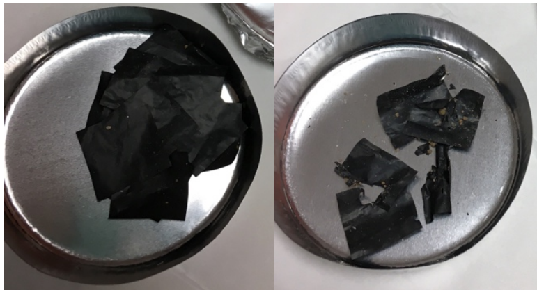
Figure III-10. Visual degradation of PLA/PHA mulch fragments at 20°C (left) and 30°C (right). Remaining PLA/PHA mulch pieces after the 16-week incubation. For scale, the diameter of the tins is approximately 70 mm. More fragmentation and decomposition visible with the 30°C pieces than the 20°C mulch pieces.
