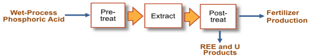
Figure 2. Conceptual Process for Recovery of REEs from Initial Produced Acid Stream
