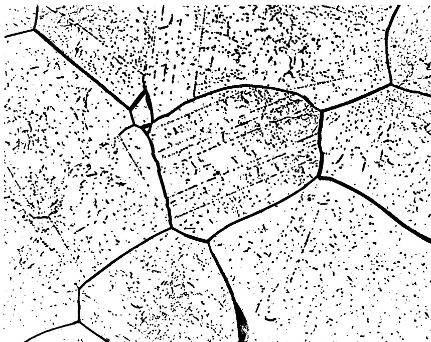
Figure IV-50. Alloy NMCR5 (3.84% Cr, 600°C, 2000 HRS.). Segmented Widmanstätten plates associated with the \beta phase. 200X.
