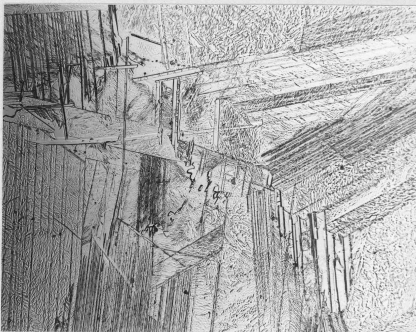
Figure IV-24. Alloy NMCR3 (0.54% Cr, 850°C, 4500 HRS.). Wavy \beta domains, secondary \alpha + \gamma G.B. reaction and \delta phase along grain boundaries. 200X.
