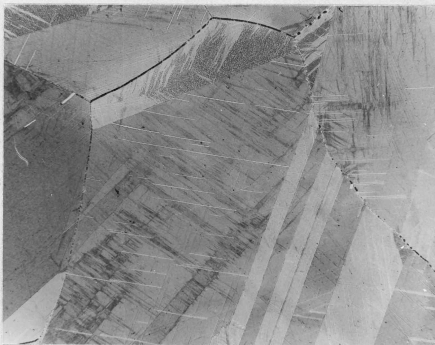
Figure IV-35. Alloy NMCR2 (2.08% Cr, 700°C, 4500 HRS.). Isolated \gamma plates in \beta matrix. 200X.
