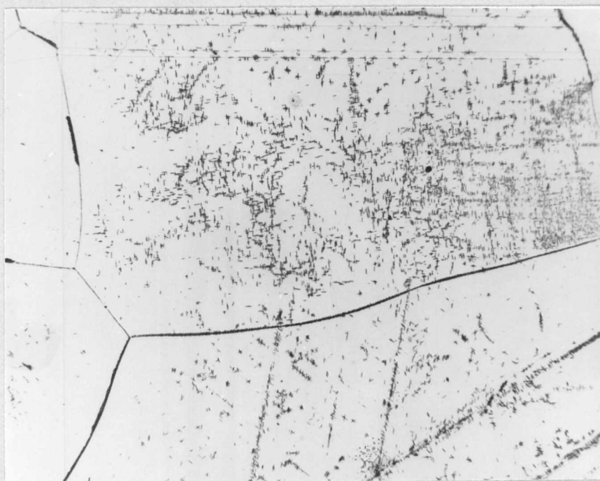
Figure IV-48. Alloy NMCR5 (3.84% Cr, 700°C, 16 HRS.). Segmented Widmanstätten plates associated with the \beta phase in \alpha matrix. 200X.
