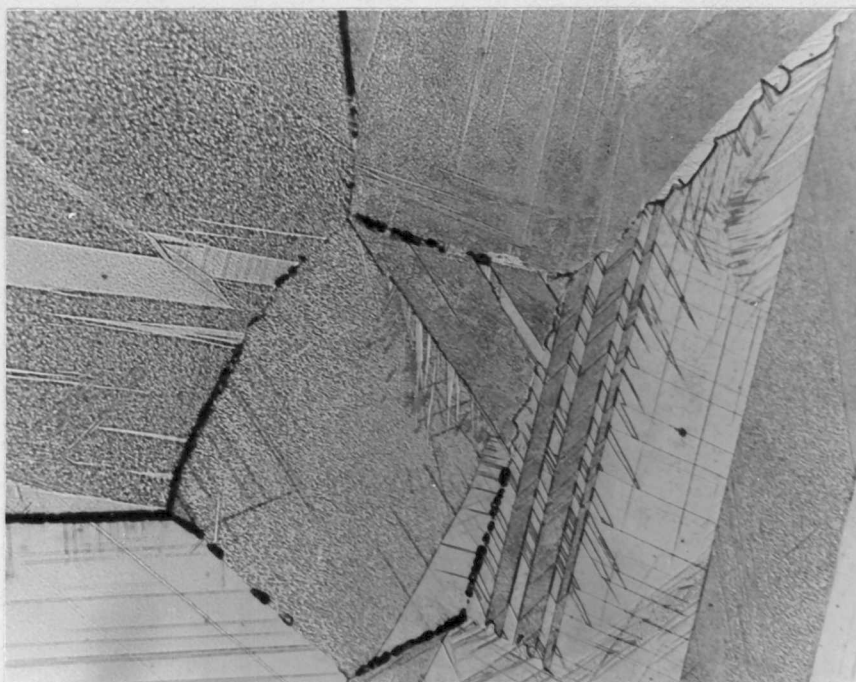
Figure IV-22. Alloy NMCR6 (0.41% Cr, 700°C, 4500 HRS.). Striations in a \beta matrix and secondary \alpha + \gamma grain boundary reaction. 200X.
