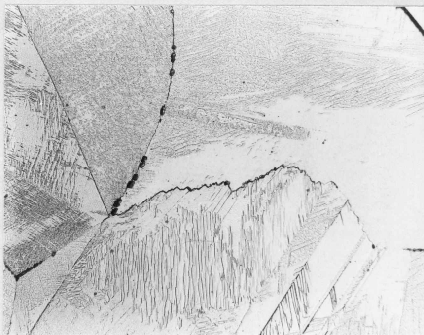
Figure IV-19. Alloy NMCRO (Ni 4 Mo, 700°C, 4500 HRS.). Tapered striations in a \beta matrix. 200X.
