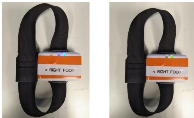
Figure 5. After turning on the sensors, LED-R will rapidly blink (for 0.1 second) “blue” or “blue and green”
