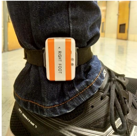
Figure 13. Foot sensor location and orientaion abobe the ankle
