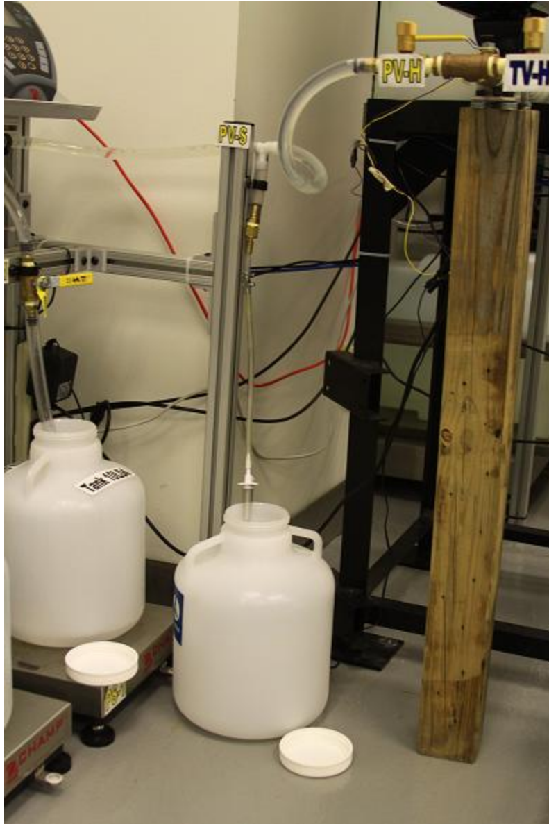
Figure A7 - Diversion Line with Collection Tank in Place
