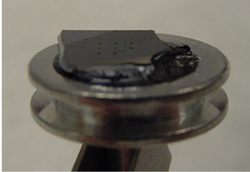
Figure 17. Polycrystalline diamond. This uncoated polycrystalline diamond sample is held at an angle. The black dots on the surface of the sample are machined features. The round carbon tape is visible under the sample.
