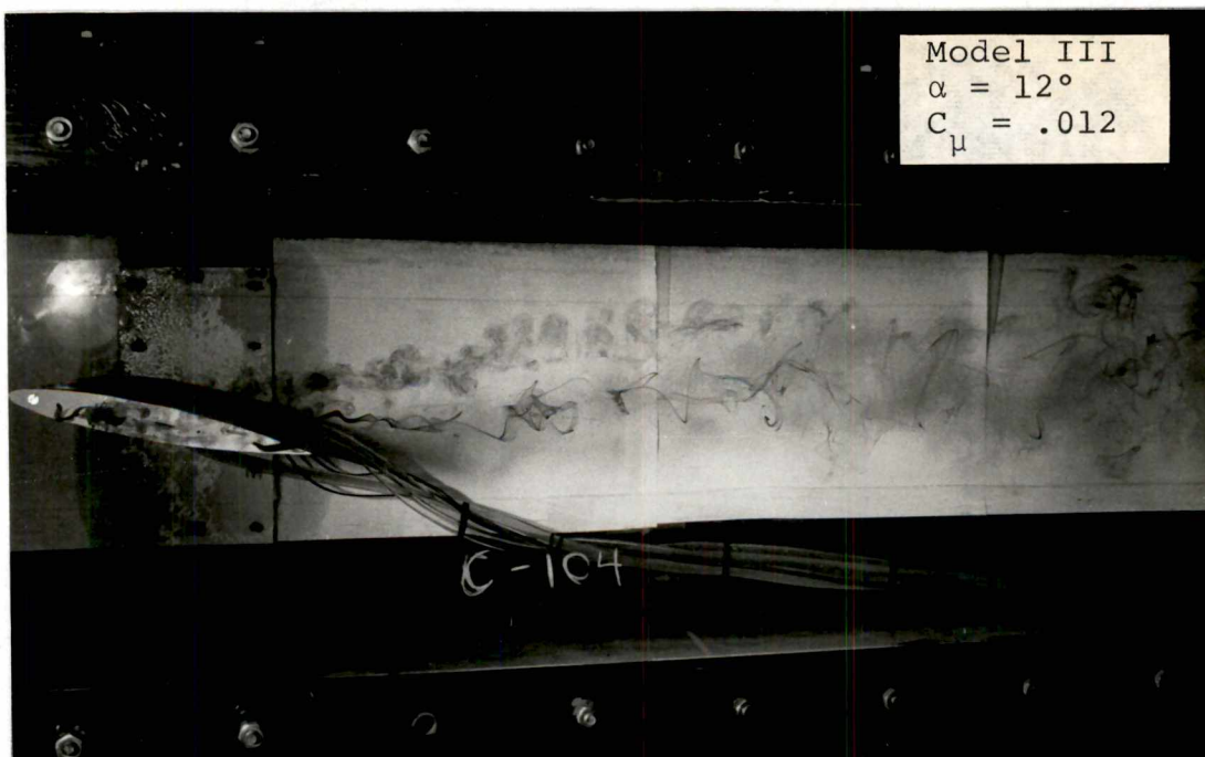
a. Front Port Blowing
