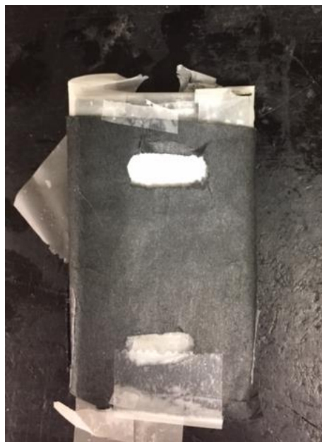
Figure 41 Photograph of the DRUV sample cell prepared inside a nitrogen atmosphere glovebox, left-without cover, right-with black cover to mask the tape.
