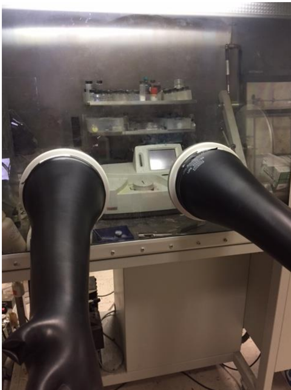
Figure 35 Photograph of the IR spectrometer located inside a nitrogen atmosphere glovebox.
