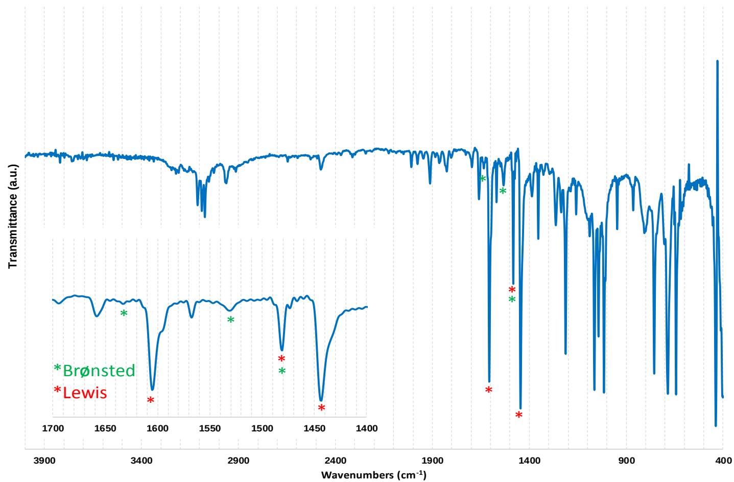
Figure 90 FTIR spectrum of \text{TiCl}_4\text{py}_2 after the first addition of pyridine (purification step). The inset is a blow up of the pyridine fingerprint region illustrating both Brønsted and Lewis pyridine are in the material.
