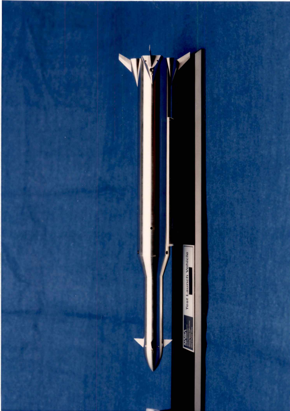
Figure B5. Fabricated test LV with fore and aft FCA's.
