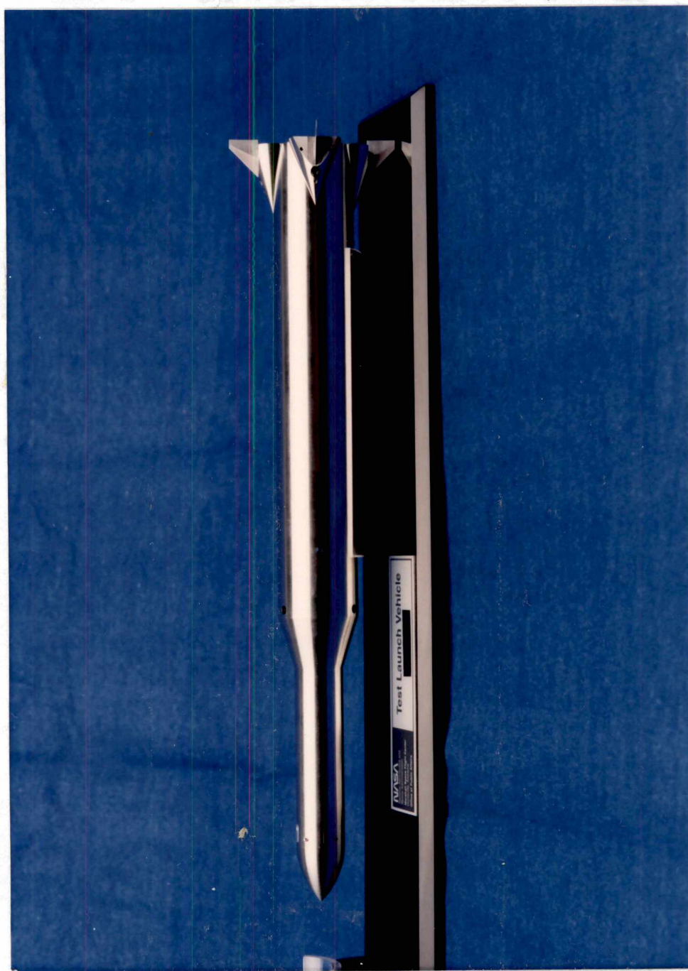
Figure 98. Photograph of fabricated test LV with aft FCA's.
