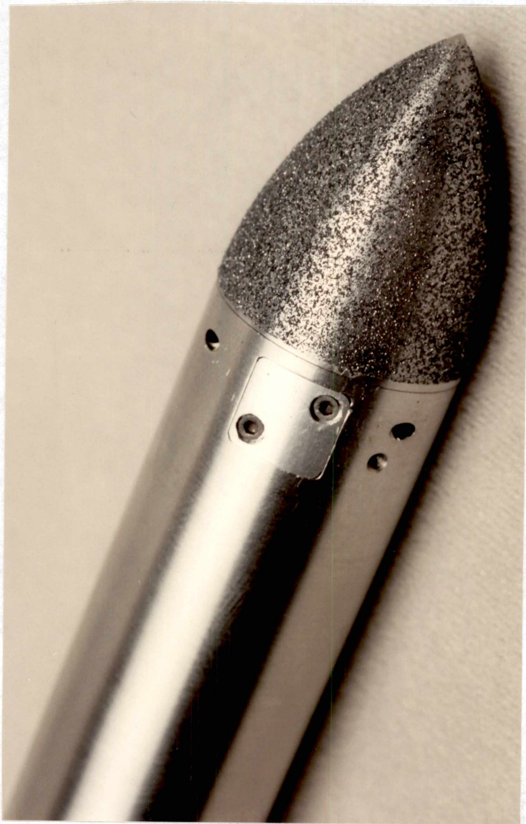
Figure B2. Nose cone silicon carbon grit size #100 applied.
