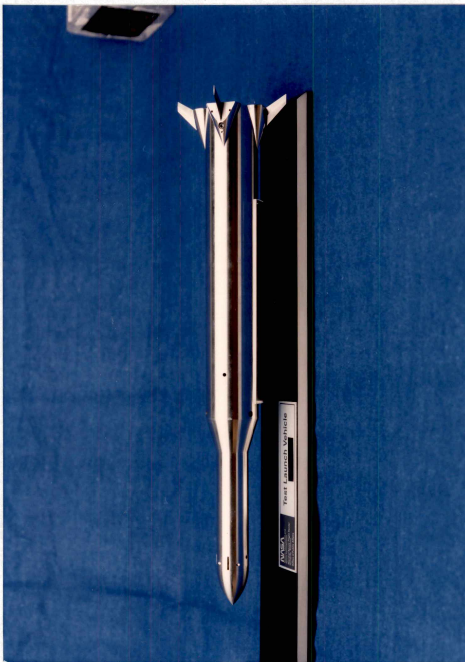
Figure B4. Fabricated test LV with FCA's #9.
