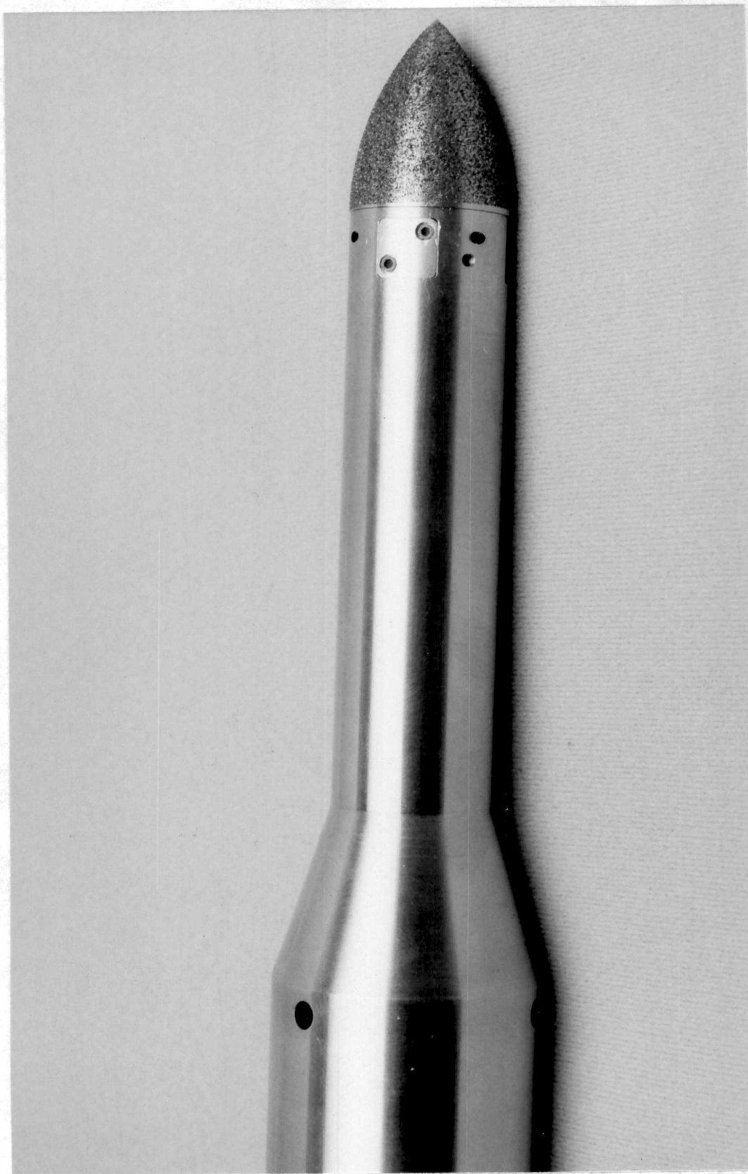
Figure B1. Silicone carbon grit size #100 applied.
