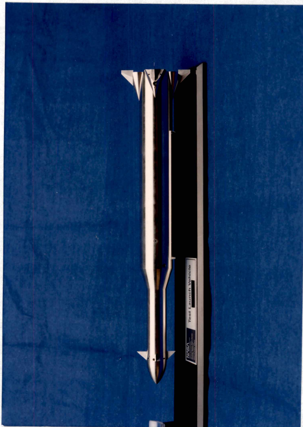
Figure 100. Photograph of fabricated test LV with canards and aft FCA's.
