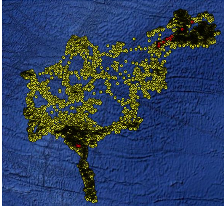
Figure 4.32. Google Earth image of entire Atlantis 9000 system buses (yellow) and buses tripped in Stage 2 (red) from tripping largest generators in Zones 5 and 21
