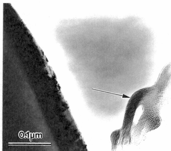
Fig. 93. A micrograph of a sample implanted at 900^\circ\text{C} with 340 keV Cr ( 4 \times 10^{16} ions- \text{cm}^{-2} ). A piece of glue which held the cross section together during sample preparation can be seen in the photograph (denoted with an arrow).
