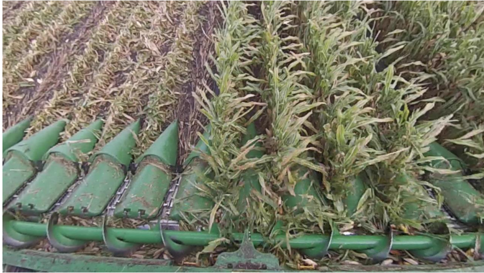
Figure 19. Example of a situation mid-field where the harvester harvested at 50% of the header capacity.
