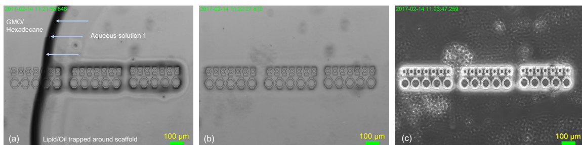
Figure 6.6: Brightfield (a, b) and phase contrast (c) microscopic images showing printed ring-type scaffolds. (Design 2 in Figure 6.1(c))
