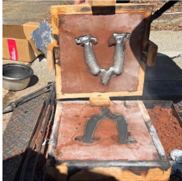
Figure 16. Single-component design after pouring in the sand mold.
