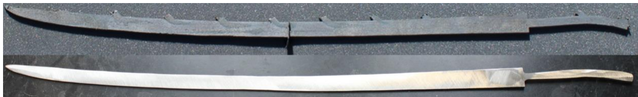
Figure 20. Blade before and after machining and finishing.
