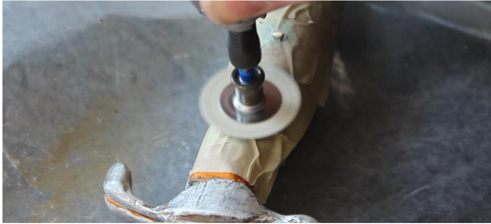
Figure 21. Brass pins being removed from the handle.
