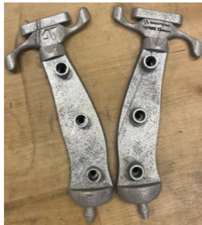
Figure 15. 3D printed scaffolding for separate-component design.
