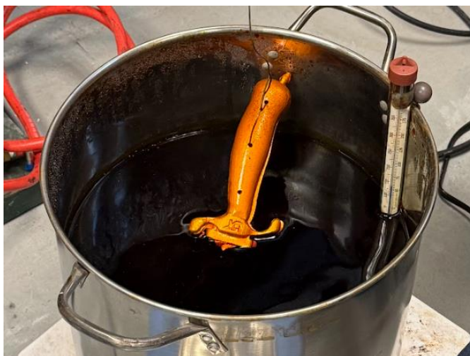
Figure 27. Anodizing of the cross guard-handle assembly.
