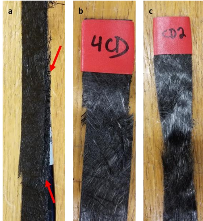
Figure S5. A) Delamination failure mode in machine direction virgin fiber composites; b) Local fiber pull-out failure mode in cross direction virgin fiber composites; c) Necking failure mode in recycled fiber composites
