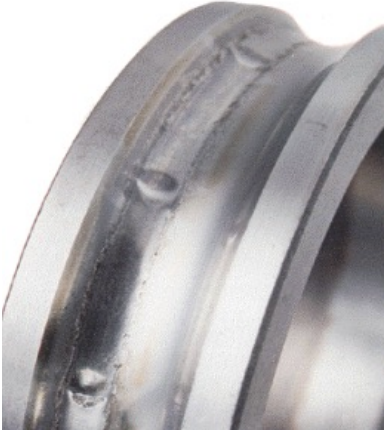
Figure 2.3. Brinelling of a ball bearing [14].
