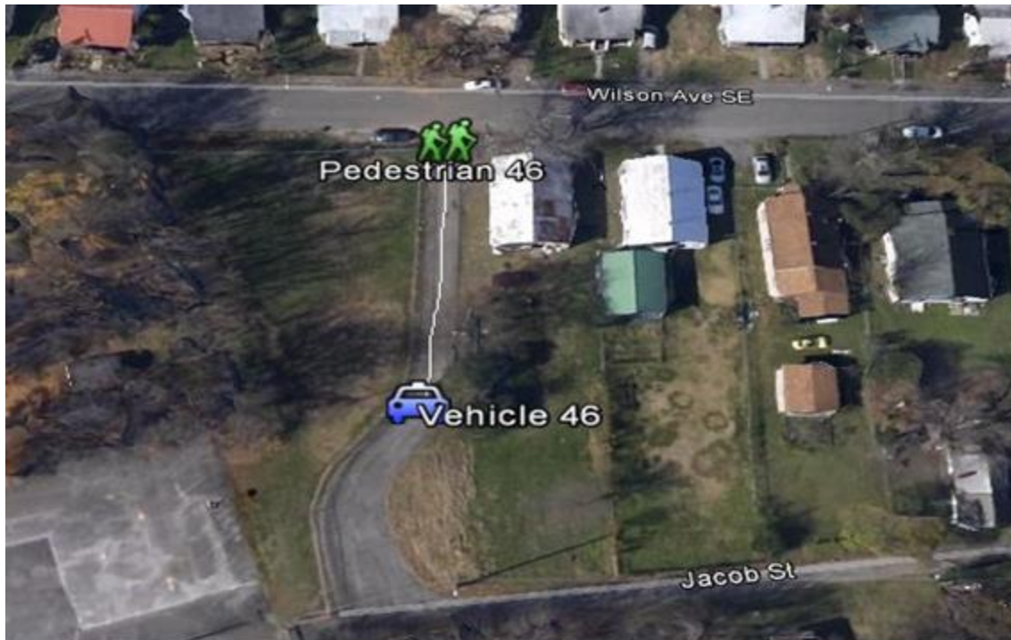
Figure 25 Stopping sight distance conflict at crosswalk at intersection of Wilson Avenue SE and 11 th Street SE
