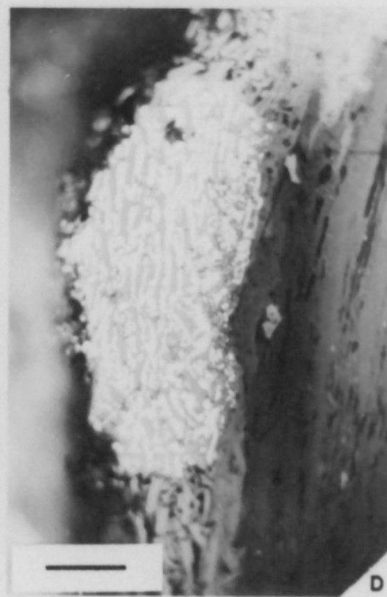
Figure 5. Reflected light photomicrographs of pyrites. (A) Framboidal pyrite seen as myriad spheres in vitrinite; (B) framboidal pyrite with compaction structures; (C) fissure-filling pyrite; (D) inertinite which has been pyritized. Scale: bar equals 70 microns.
