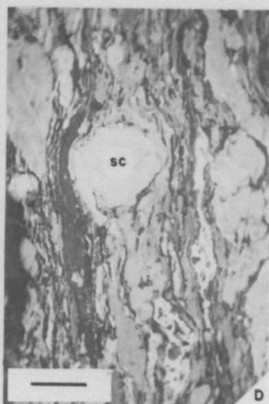
Figure 9. Reflected light photomicrographs of sclerotinite and inertinite with exinite which suggests dry conditions in the swamp. (A) Inertinite and exinite; (B) sclerotinite in vitrinite with reflectivity decreasing away from the sclerota; (C) unusually well-preserved tellinite and collinite which grade into inertinite; (D) sclerotinite and exinite with little or no vitrinite. Scale: bar equals 70 microns.
