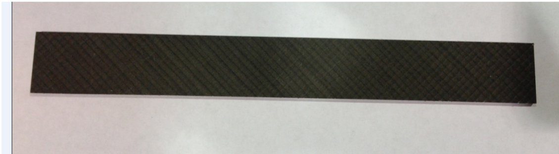
Figure 4.2: Image of 25.4 mm length x 200 mm width x 2.8 mm thick [ \pm 45 , 2s] carbon fiber with vinyl ester resin (CFVE) tensile sample.
