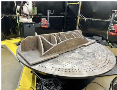
Figure 24. Final product at 77% completion. Notice the warpage between the part and the build table.
