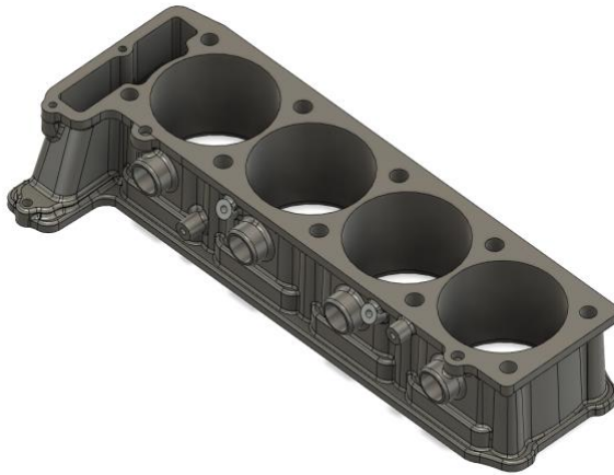
Figure 13. CAD model derived from the SLS scan of the original Mitsubishi engine block.
