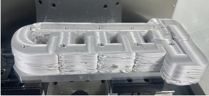
Figure 17. Preform post three-axis milling. Notice the predrilled holes coming out of the bottom surface. The fiducial stickers are left over from SLS process.
