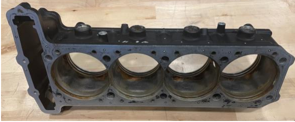
Figure 11. Original Mitsubishi engine block with fiducial stickers utilized in the SLS scan.
