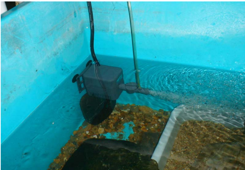
Figure 12: Powerhead being used to create circulation.
