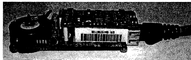
Figure 2: Previous Wired Geiger Mueller Sensor Packages
