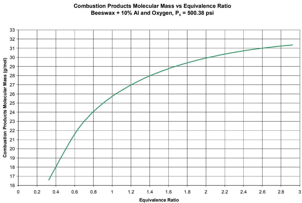
Figure 93: Molecular Mass vs. Equivalence Ratio, Beeswax + 10% Al/Oxygen, P_c = 500.38 psig
