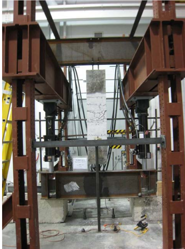
Fig.4.9. Tension test set-up
