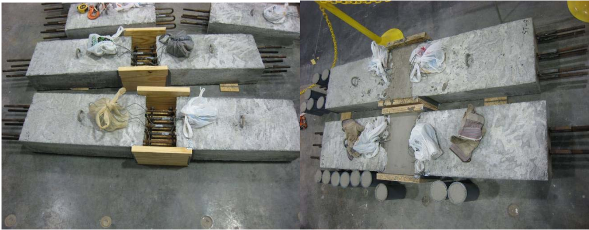
(a) Before grouting
