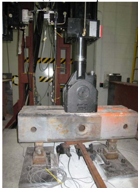
(b) Apparatus applying fatigue forces
