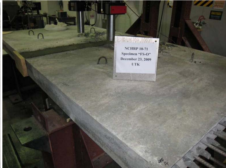
(b) After grouting
