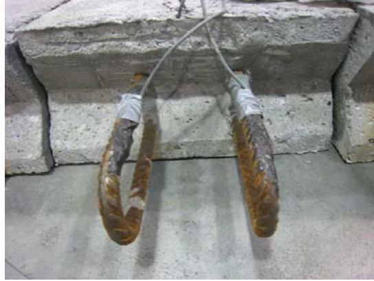
Fig.4.7. Profile of joint surface after sandblasting
