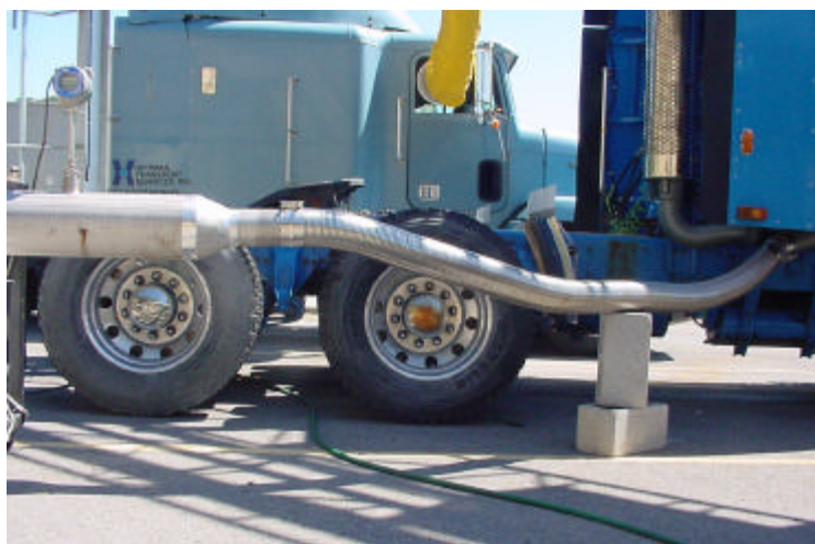
Figure 3.2. Test truck attached to primary sampling chamber.
