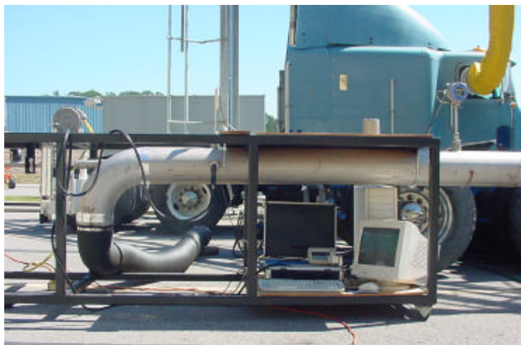
Figure 3.4. Side view of primary sampling chamber.
