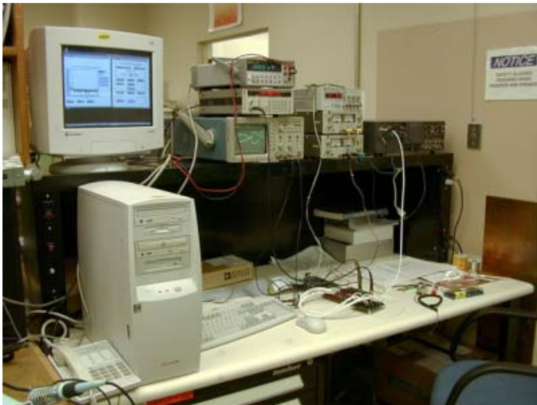
Figure 7.6 Photograph of modulator test & characterization system.
