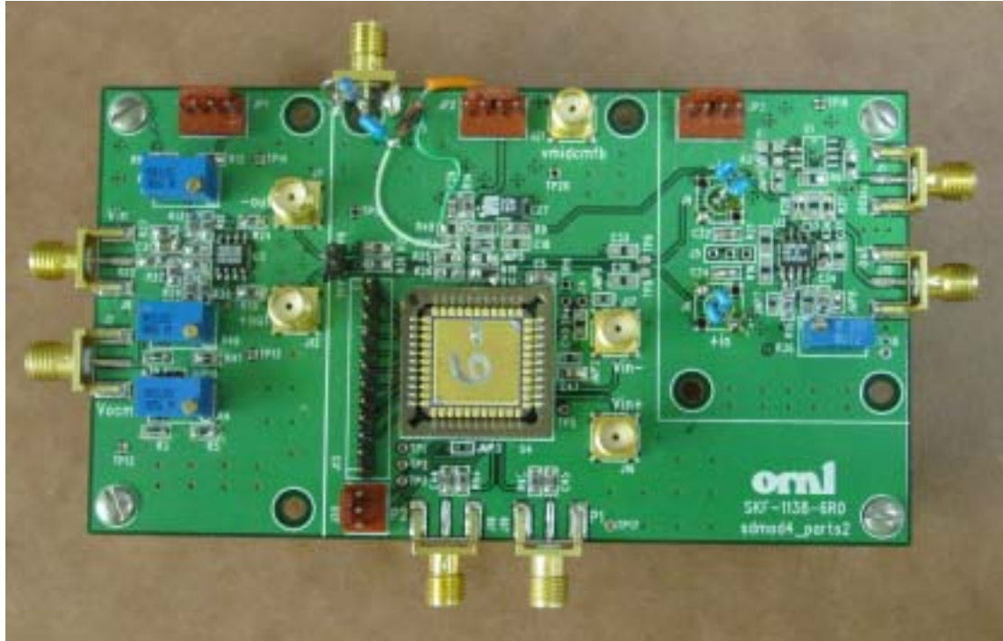
Figure 6.4 Photograph of modulator components test PCB.
