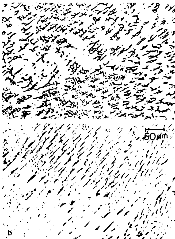
FIGURE 7. AS-WELDED OPTICAL MICROSTRUCTURES. (a) ARGON SHIELDED: (b) ARGON-NITROGEN SHIELDED
