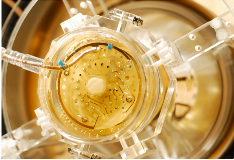
Figure 6.10: Picture of the DC inner detector PMT base.
