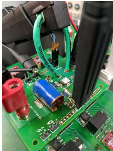
Figure 4.23 Prototype 15-mil, 6 nH air core inductor
